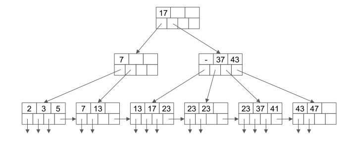
• If an interior node has keys  $K_1, K_2, ..., K_n$ , then  $K_i$  is the smallest *new* key that appears in the part of subtree accessible from the (i + 1)st pointer
