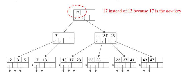
• If an interior node has keys  $K_1, K_2, ..., K_n$ , then  $K_i$  is the smallest *new* key that appears in the part of subtree accessible from the (i + 1)st pointer
