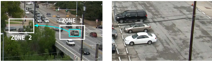
(a) MIRIS [11] requires hardcoded zonal markings to detect a left turn.
