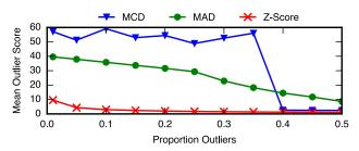
Figure 3: Discriminative power of estimators under contamination by outliers (high scores better). Robust methods (MCD, MAD) outperform the Z-score-based approach.
