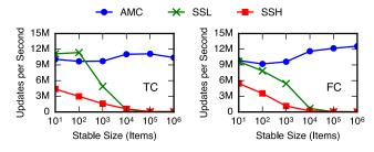
Figure 6: Streaming heavy hitters sketch comparison. AMC: Amortized Maintenance Counter with maintenance every 10K items; SSL: Space Saving List; SSH: Space Saving Hash. All share the same accuracy bound. Varying the AMC maintenance period produced similar results.
