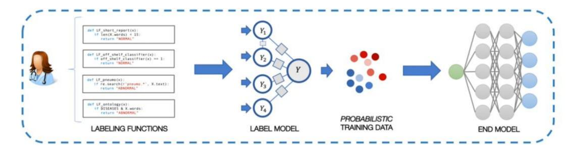
(1) Users write labeling functions to generate noisy labels (2) A label modelcombines noisy labels tobe probabilistic labels
